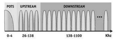
The number of bits per channel depends on the properties of the line (Line Gain) as it can be seen in the following illustration. Subbands, which have high noise problems, can be avoided to guarantee a proper transmission.
